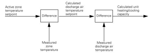
If the discharge air temperature falls below the Discharge Air Control Point Low Limit (configurable using the Rover service tool) and cooling capacity is at a minimum, available heating capacity will be used to raise the discharge air temperature to the low limit (see "Discharge air tempering" on page 39).
